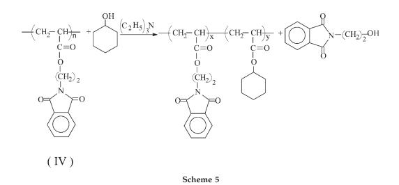
For equivalent quantities of polymer, cyclohexanol, and triethylamine, the progress of the reaction<sup>5</sup> (percent exchange) was recorded against the reaction time (*t*) at 20 and 60°C. The results are reported in Tables V and VI. From Tables V and VI, it is clear that poly-NPEA showed a good behavior as a model compound for a long-active polymeric drug (Scheme 5).
